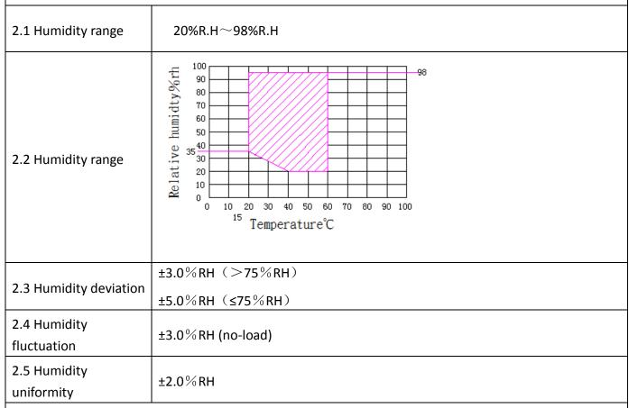
Temperature and humidity performance test is in accordance with the relevant provisions of the IEC60068 -3 standard measurement; sensor placed in the unit outlet.
